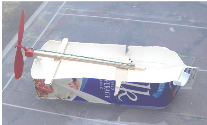
Rubber band powered boat using “nose hook” propeller from an airplane model.
